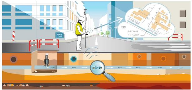
The GeoBot partners are building a small robot (think of a matchbox-sized RC car) that will be inserted into a gas pipe, and move around it to map the location of the different underground pipes. Such mapping is necessary to prevent gas-related accidents, for example during construction. At the end of the project, this solution will be commercialized and used to map the network of gas pipe in France, before being used in worldwide.
